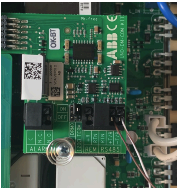
RS485 terminals on the ABB/FIMER UNO-DM-COM KIT expansion card
